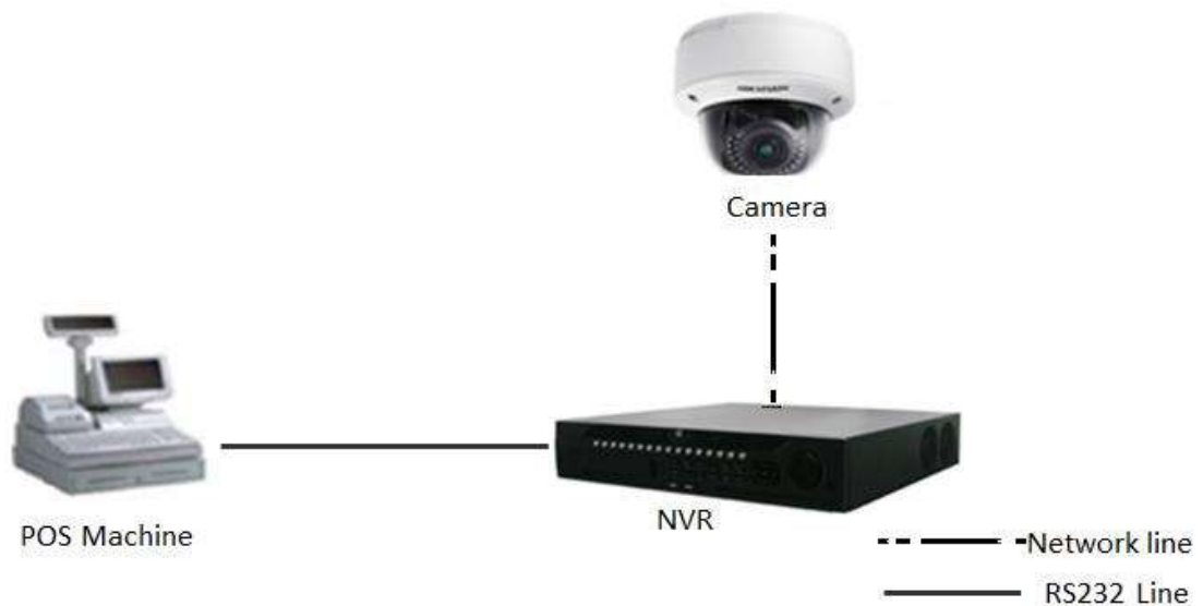
Rys. 14 Topologia RS-232 POS z DVR
